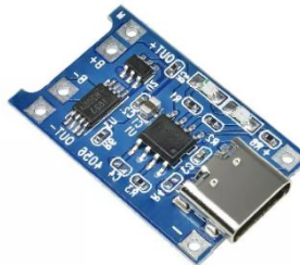
Figure 34: Circuit de charge TP4056
