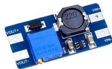
Figure 35: Circuite booster MT3608
