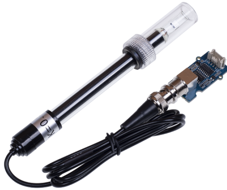
Figure 3.9: Electrical conductivity meter
