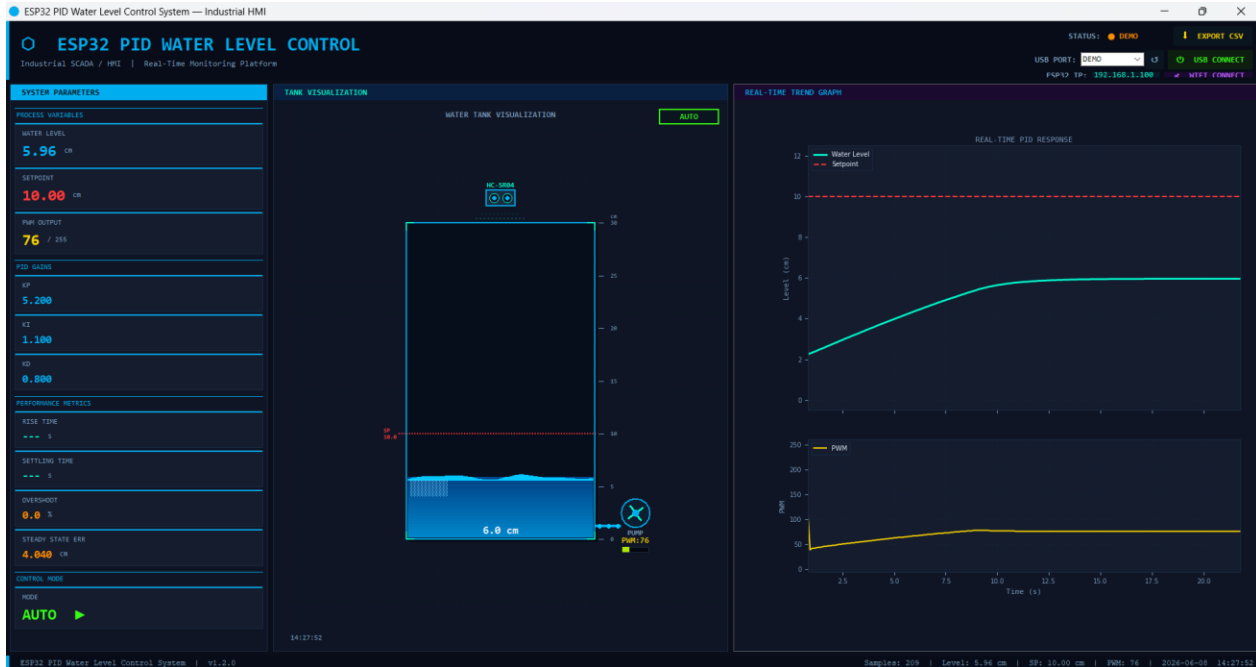
Figure 24 Python SCADA Monitoring Application (v04.py)
