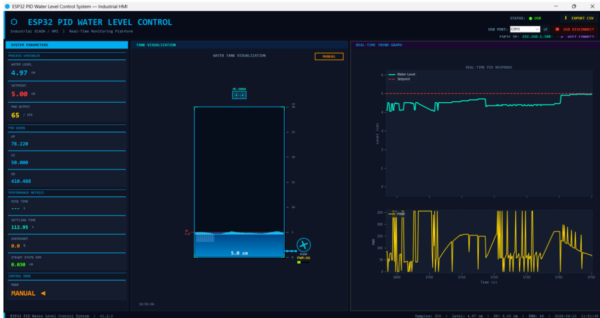
Figure 32:: Level response — Manual mode with increased Ki (enhanced integral action)
