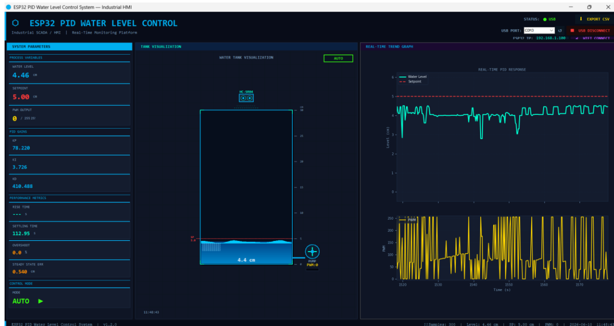
Figure 30: Level response — Auto-Tuning Trial 3 (Auto mode, setpoint 5 cm)
