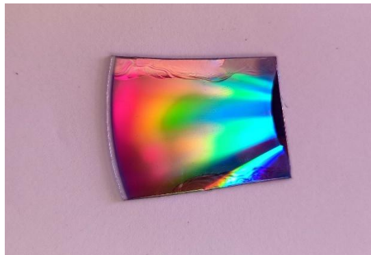
Figure 28: DVD piece containing microscopic grooves.
