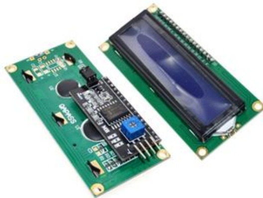
Figure 32 : Afficheur LCD I2C (16)
