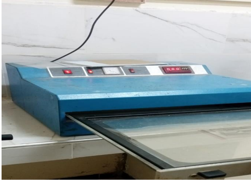
Figure 93: Circuit Printer on Copper Plate
