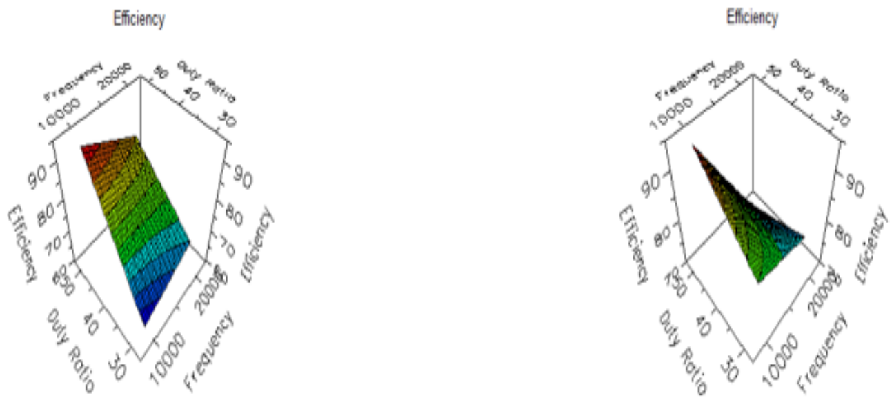
Figure 52 : Response surface in the case of a low and high resistive load
