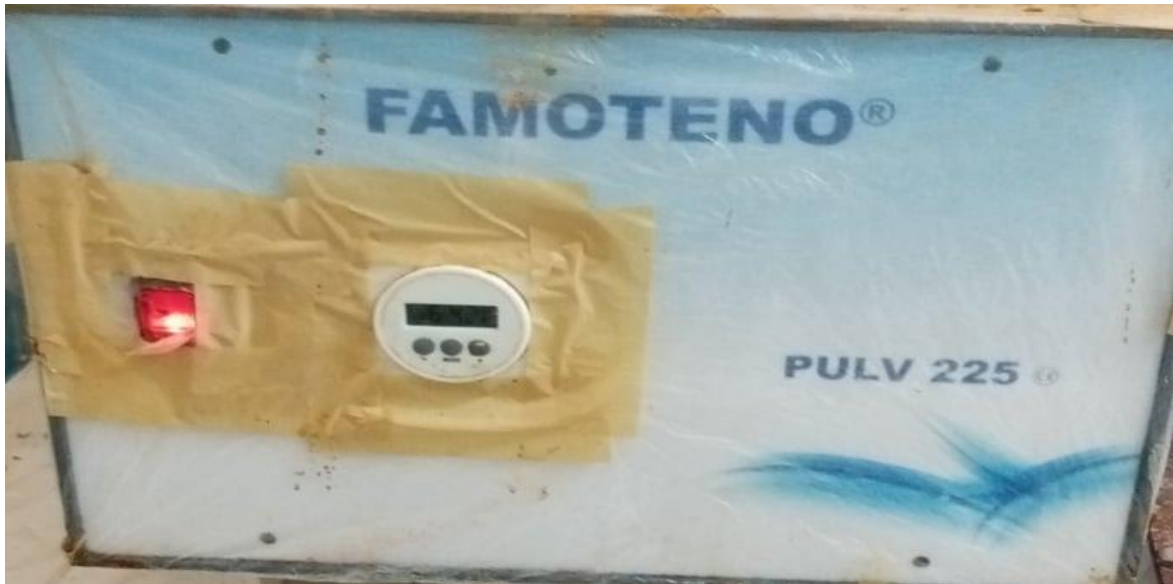
Figure 95: Machine for Copper Removal from the Plate
