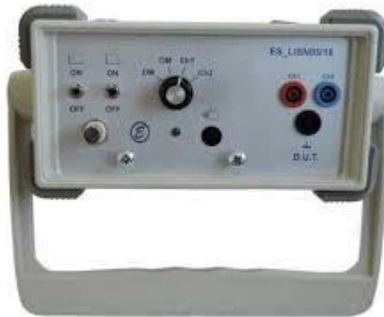
Figure 63 : A Line Impedance Stabilization Network (LISN)
