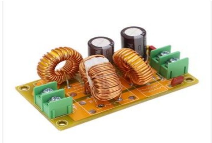
Figure 26: LC Filter in PCB
