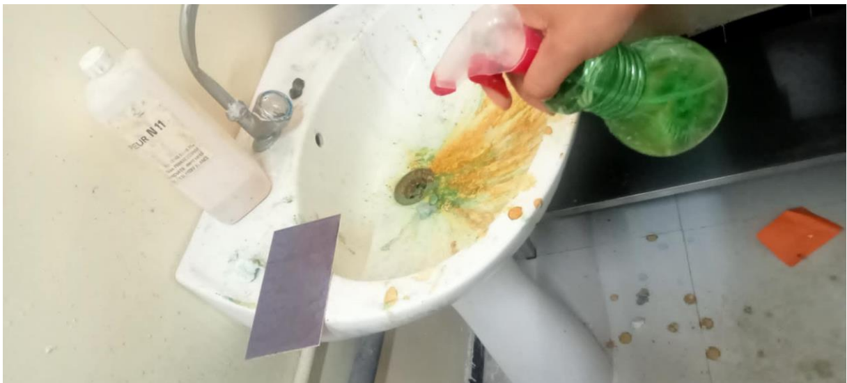
Figure 94: Washing the Plate to Reveal the Circuit
